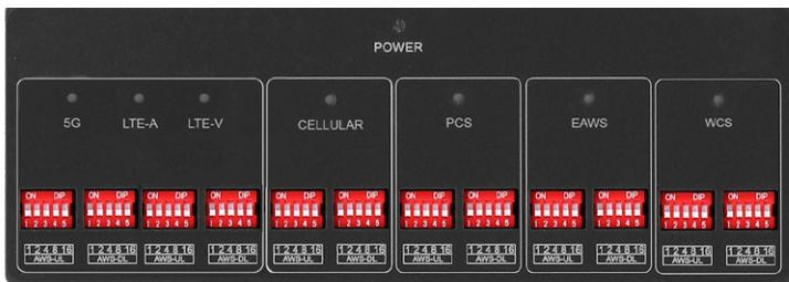
Switches should be OFF unless flashing red/yellow flashing lights occur for a channel or channels. Red/yellow flashing lights indicate the system has detected oscillation for the corresponding channel(s). They then turn off if adjustments are not made. When adjusting the booster, full power is not always the best option. Your goal is to obtain a usable signal in as many areas of the building as possible.
