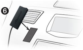
Identify a location for the inside antenna on or near your front dashboard that is: (1) Within 2-3 feet of typical cell phone location, (2) At least 8 inches (20cm) from cellular devices and (3) At least 4 inches (10cm) from metal.
