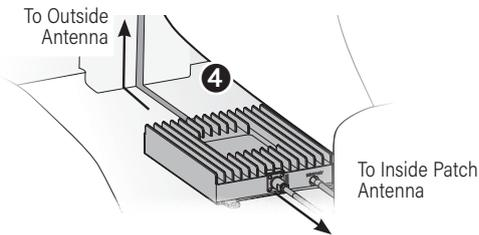
Select a well-ventilated location for the booster that is away from excessive heat, direct sunlight, and moisture. Beneath a seat or within the front console is suggested.
