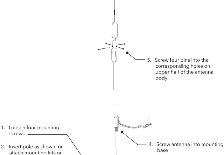
3. Tighten all four screws in place and secure with wrench
